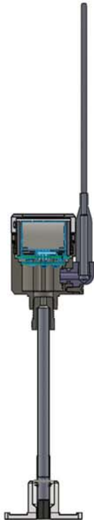
Cross-sectional view of high-temp dual-element microPIMS® sensor.
